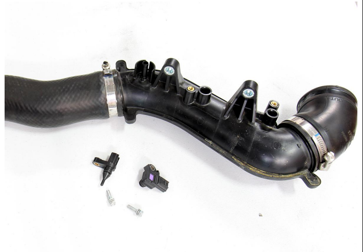
17. Use an 8mm socket to remove the IAT and MAP sensor from the factory charge pipe.
