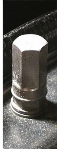
**STEP 7** - Slide open the red positive cover on the battery. Clip the red (positive) battery clip (B) onto the tab underneath the red cover. Clip the black (negative) battery clip (B) onto a nearby ground stud such as the one pictured to the right.
