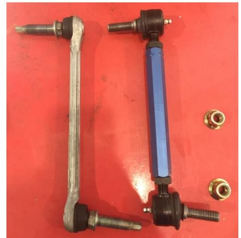
Figure 2: Factory vs Steeda front swaybar endlinks
