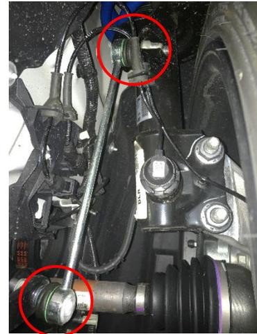
Figure 1: Factory front swaybar endlink
