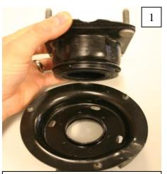
Separate the bearing and bushing from the spring seat itself with a screwdriver
