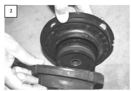
4. Remove the spring seat base from the new assembly. Insert the new spring base into the factory rubber spring seat. Be sure to keep the billet spring seat base face up to prevent disturbing the bearing inside. **Pics 3 & 4**
