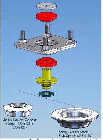
Note: The installation of these Competition Upper Strut Mounts requires the removal of the factory mounts that have the springs in a preloaded state. The potential energy stored in the springs can be very dangerous if not properly disassembled. Follow the factory service procedures or have this installation performed by a qualified technician. It is recommended that a factory service manual be available when installing these new mounts. The provided grease is used for the urethane bushings only!
