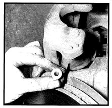
5 Start the new stainless sleeve from the pad side of the caliper. Lightly lube the O.D. with high-temperature grease first to assist driving it into the bore. To get the sleeve started, give a few light hammer taps around its circumference. You want the sleeve to start straight.
