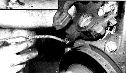
**7** Dry fit the caliper pins. If they slide through, great. If not, you'll have to drill the sleeve I.D.s. What's happened is the sleeve has taken on the sometimes out-of-round shape of the caliper holes, pinching the sleeve I.D.s. Before drilling the sleeves, lube them with cutting oil.
