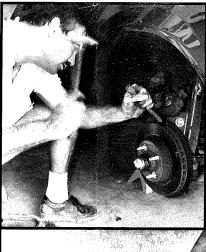
**6** Once the sleeve is started, drive it home with a hammer and drift. A soft drift, such as brass or even wood, is required. A steel drift can displace the steel sleeve, causing a ding which will need filing before the pins will pass through.
