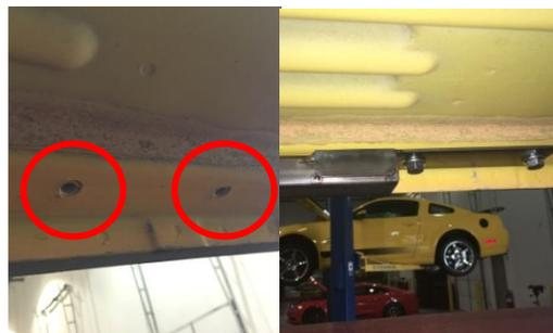
Figure 4: Steeda chassis jacking rail (rear)
