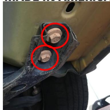
Figure 1: Factory front cross brace bolts
