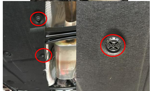
Figure 2: Underside panel hardware
