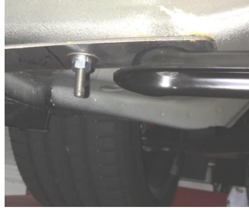
Figure 5: Steeda jacking rail front bracket
