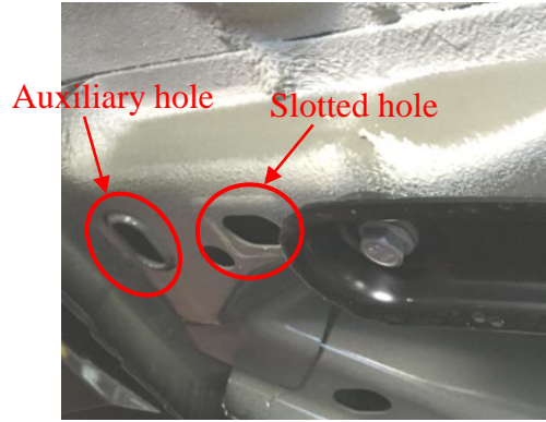
Figure 4: Slotted and auxiliary hole for offset stud
