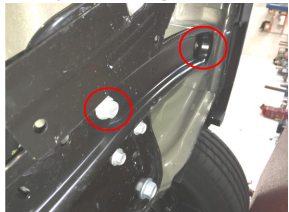
Figure 3: Cross brace bolts
