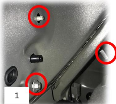
Figure 1: Factory taillight nuts
