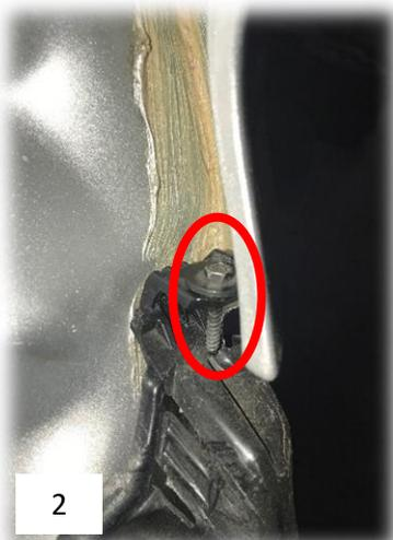
Figure 2: Top bolts on rear bumper
