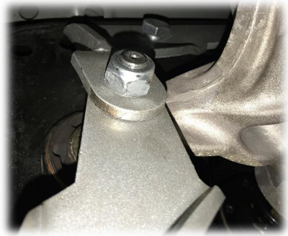
Figure 3: Steeda THRU threaded differential bolt and nut configuration (shown with Steeda's 555-4050 Differential Brackets)
