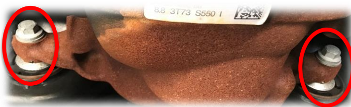
Figure 2: Front differential bolt locations
