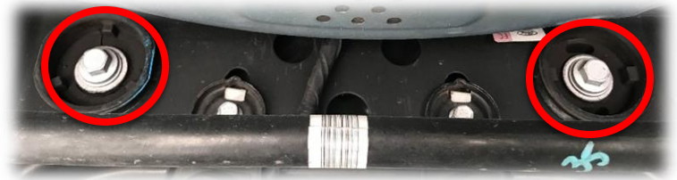
Figure 4: Rear differential bolt locations
