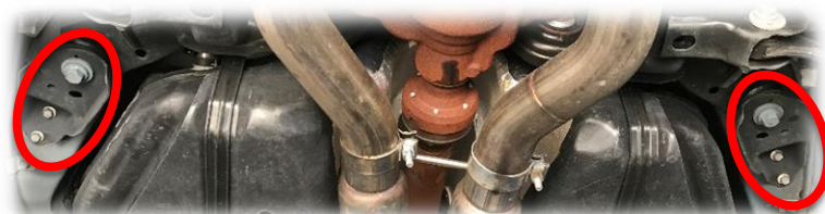
Figure 1: Main subframe and subframe support bracket bolt locations
