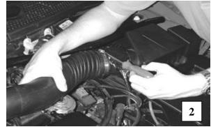
Disconnect the factory intake tube from the filter box. Loosen the hose clamp by the mass air meter and separate the tube from the air box. (Pic 2)
