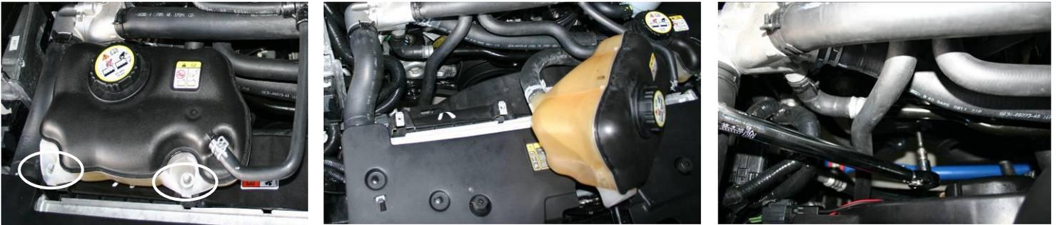
3. Remove the 3 coolant outlet bolts circled in the picture.
