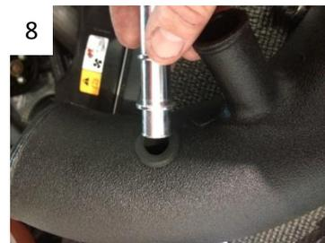
8. Remove the factory air intake sensor. This is located in the factory lid facing forward. Simply rotate it counter clockwise to remove. Use the supplied rubber grommet (smaller OD) and install the grommet into the forward facing hole in the Steeda CAI base. Then using a twisting motion install the sensor as shown. See figure 5.
