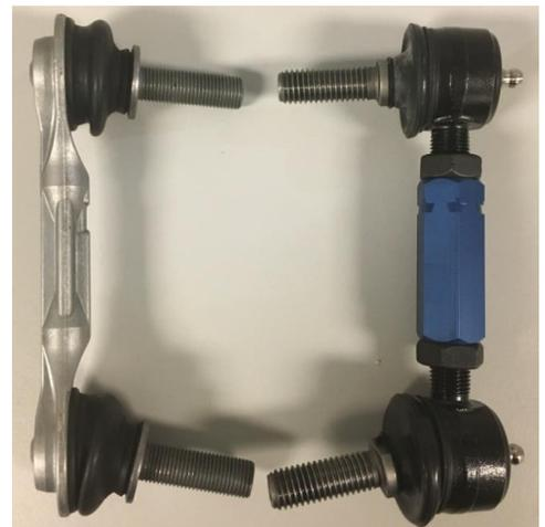
Figure 2: Factory vs Steeda rear swaybar endlinks
