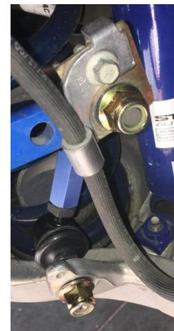
Figure 3: Steeda adjustable rear swaybar endlinks
