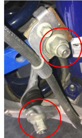
Figure 1: Factory rear swaybar endlink
