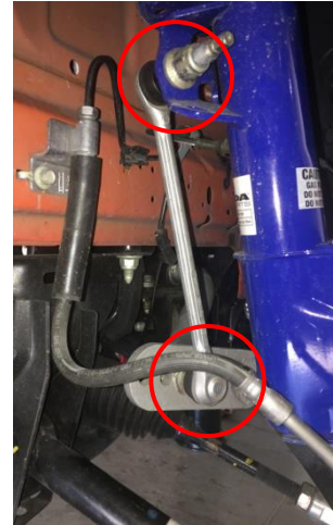
Figure 1: Factory front swaybar endlink
