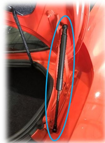
Figure 1: Factory trunk struts
