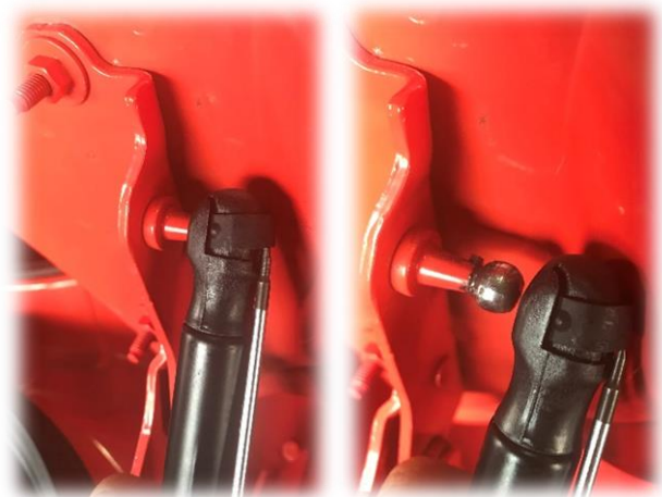
Figure 2: Strut removal process
