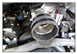
13. Install the provided coupler onto the throttle body and secure with the provided hose clamp. Tighten clamp using 5/16" socket or nut driver. **NOTE: Do not over tighten clamps.**
