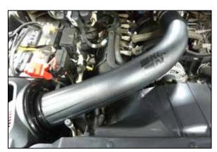
15. Install the K&N intake tube into the filter and then into the coupler at the throttle body, adjust for best fit and then secure with the provided hose clamps. Tighten clamps using 5/16" socket or nut driver. **NOTE: Do not over tighten clamps.**
