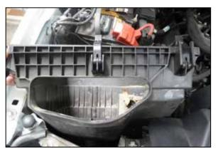
8. Pull up the lower air filter housing to dislodge it from the mounting grommets and then remove it from the vehicle.
