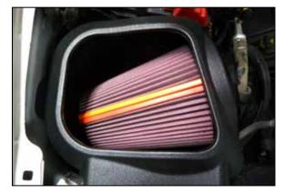
12. Install the K&N air filter into the K&N air filter housing.
