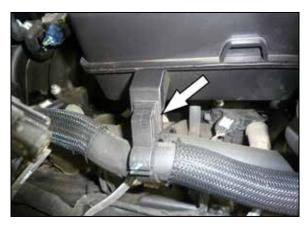
4. Disconnect the vent line holder from the factory intake plenum.
