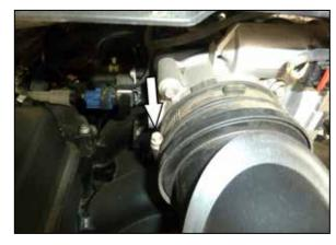
5. Loosen the hose clamp that secures the intake plenum to the throttle body. Remove the complete intake tube and plenum assembly from the vehicle.
