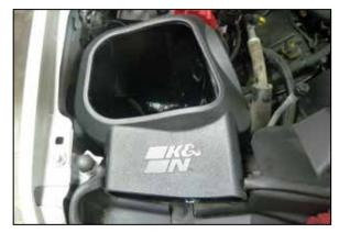
10. Install the K&N air filter housing and secure with one of the factory bolts from step #9.
