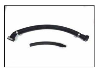
16. Install the provided quick connect fittings into the provided CCV hose and secure with the provided hose clamps. Install the union fitting into the EVAP hose.
