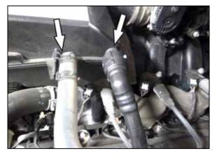
3. Disconnect the two vent lines from the factory intake plenum.
