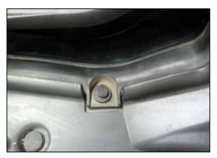
6. Remove the push-pin that secures the fresh air duct to the core support and then remove the duct from the vehicle.
