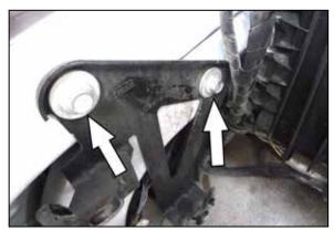
9. Remove the two bolts that secure the factory air filter housing mounting bracket to the inner fender and then remove the bracket from the vehicle.
