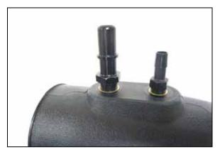
14. Install the provided vent fittings into the K&N intake tube as shown.
