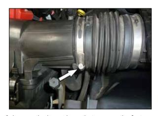
2. Loosen the hose clamp that secures the factory intake tube to the air filter housing.
