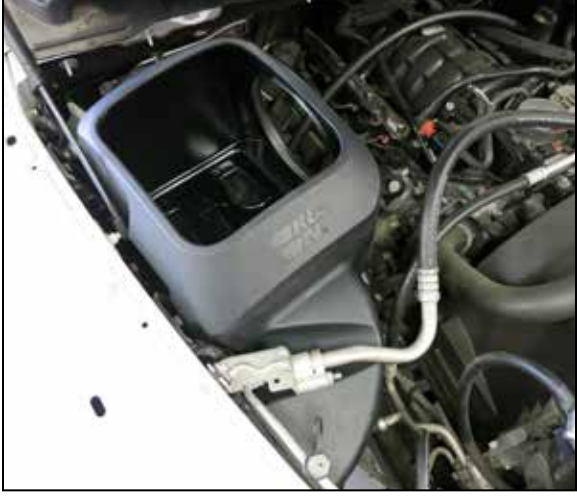
11. Install the K&N air filter housing into the vehicle so the mounting posts protrude through the mounting grommets.
