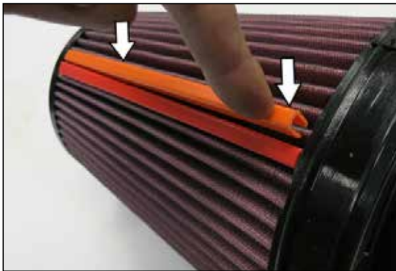
12. Attach the filter clips to the pleats on the air filter align and push down. Passenger side filters, place orange clip on top and red on bottom.
