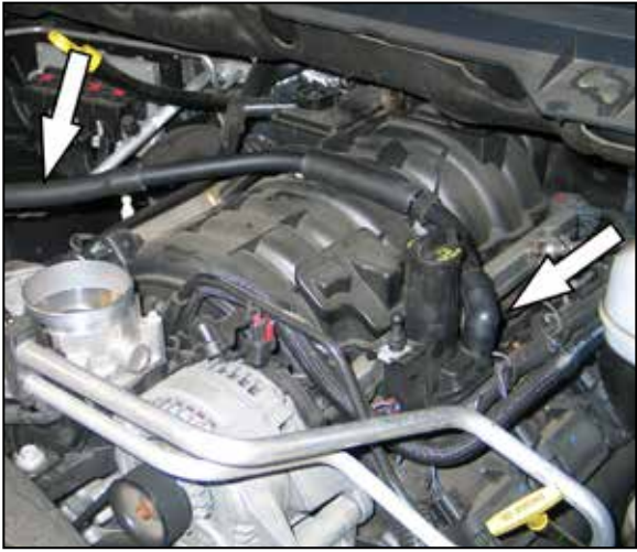
6. Remove the complete CCV hardline assembly from the valve cover.
