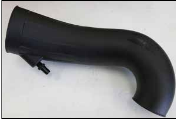
14. Install the provided CCV fitting into the K&N intake tube. NOTE: The CCV fitting utilizes 3/8npt threads, hand tighten and then tighten one revolution with the appropriate size wrench.
