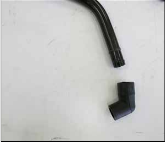
7. Remove the elbow from the plastic hardline.
