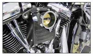
6. Install the K&N® servo cover and secure with the provided hardware to the original servo cover mounting bolt locations.
