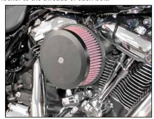
14. Install the top plate onto the filter and secure with the provided hardware.
