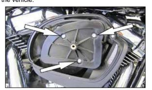
3. Remove the three bolts that secure the air filter element and then remove the air filter and crank case breather tubes.
