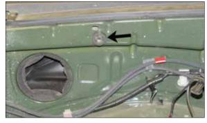
13. Install the 6mm rubber mounted stud into the inner fender location shown.
