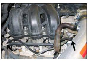
28. Connect the provided fuel pressure vent line to the fuel pressure regulator and then connect the open end to the 3/16 vent fitting in the K&N<sup>®</sup> intake tube.
