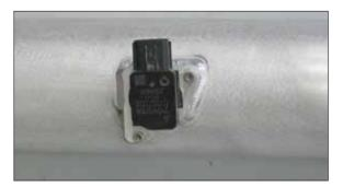
23. Install the mass air sensor into the K&N<sup>®</sup> intake tube and secure with the provided hardware.
