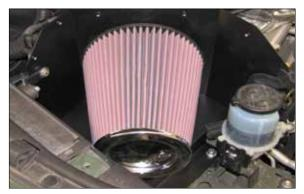
29. Install the K&N<sup>®</sup> air filter onto the filter adapter and secure with the provided hose clamp. NOTE: Drycharger<sup>®</sup> air filter wrap; part # RF-1020DK is available to purchase separately. To learn more about Drycharger<sup>®</sup> filter wraps or look up color availability please visit http://www.knfilters.com<sup>®</sup>.
