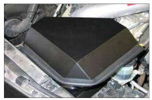
31. Install the heat shield cover onto the heat shield and secure with the provided hardware. NOTE: Use of the heat shield cover is not mandatory; it is recommended that the cover is used during conditions of heavy moisture such
