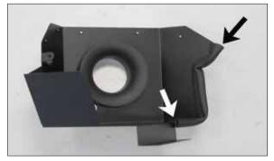
18. Install the 10.5" long piece onto the heat shield as shown.
