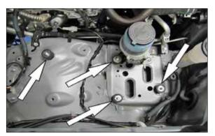
12. Install the four rubber mounted studs into the factory air box and P/S reservoir as shown. NOTE: The forward most rubber mounted stud is only used if the vehicle is equipped with the air injection pump located in front of the factory air box.
