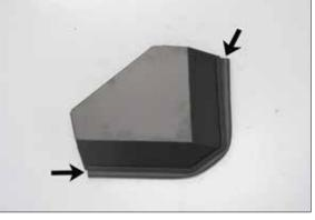
30. Install the remaining 19" piece of edge trim onto the heat shield cover as shown.
