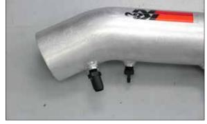
25. Install the 3/16 vent fitting into the  $K\&N^{\otimes}$  intake tube as shown.
