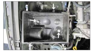
9. Loosen and remove the three bolts securing the lower air box and then remove the lower air box from the vehicle.
