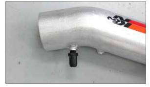
24. Install the 5/8 vent fitting into the  $K\&N^{\circledast}$  intake tube as shown.
