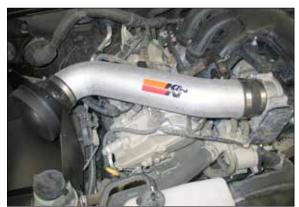
26. Install the K&N<sup>®</sup> intake tube into hump hose at the filter adapter and then into the silicone hose at the throttle body, align the tube for proper fit and then tighten the hose clamps.
