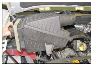
6. Pull up the air box to release it from the mounting grommets and then remove the factory air box from the vehicle.
