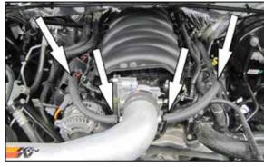
19. Connect the provided crank case vent hoses to the ports on the valve covers and then connect the open ends to the fittings installed into the K&N® intake tube and secure with the provided hose clamps.
