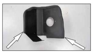
8. Install the provided edge trim onto the heat shield as shown.
