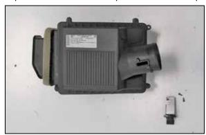
15. Remove the mass air sensor from the factory
