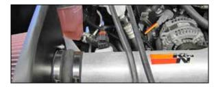
20. Reconnect the mass air sensor electrical connection.
