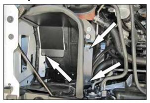
9. Install the heat shield assembly and secure to the air box mounting plate location using the three factory bolts from step #7.
