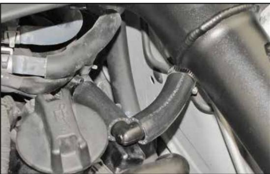
25. Connect the end of the crank case vent hose with the hose clamp to the 90° vent fitting on the driver's side K&N® intake tube and then connect the other end to the vent port on the valve cover.
