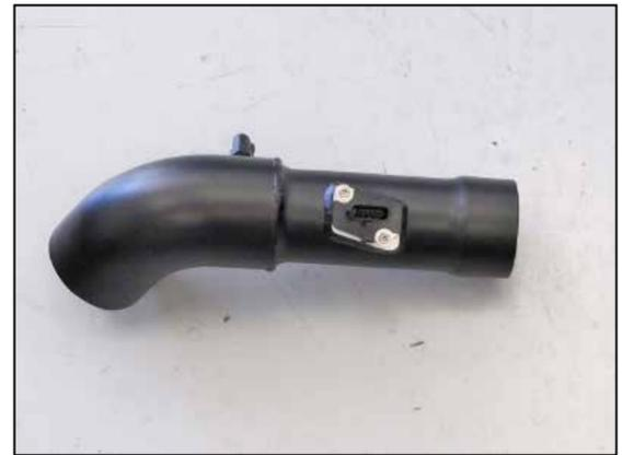
21. Install the mass air sensor into the driver's side K&N® intake tube and secure with the provided hardware.
