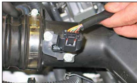
3. Disconnect the passenger side mass air sensor and unhook the wiring harness from the air box.
