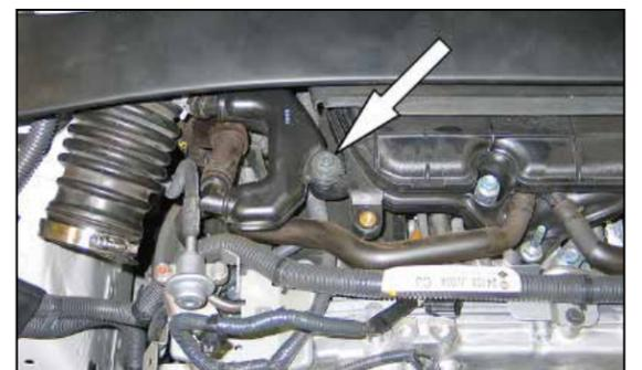
6. Remove the bolt shown which secures the crank case vent tube assembly to the intake plenum.
