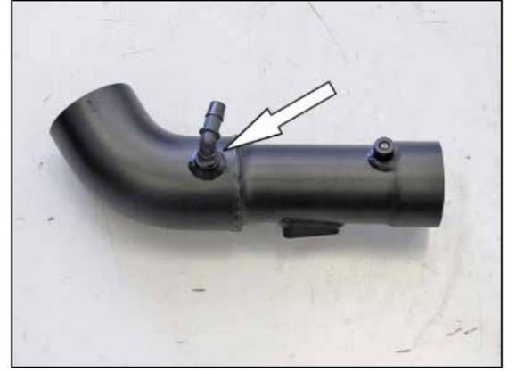
19. Install the provided 90° NPT vent fitting into the driver's side K&N® intake tube (27466) as shown.
