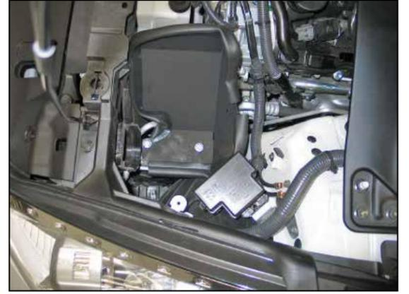
18. Install the heat shield assembly into the vehicle so that the mounting pins engage into the air box mounting grommets.
