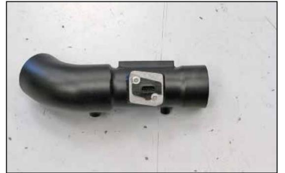
35. Install the mass air sensor into the passenger side K&N® intake tube and secure with the provided hardware.
