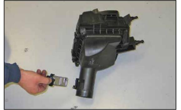
34. Remove the two screws securing the mass air sensor to the air box and then remove the mass air sensor from the air box.
