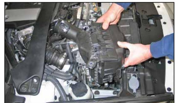
5. Remove the passenger side air box from the vehicle.
