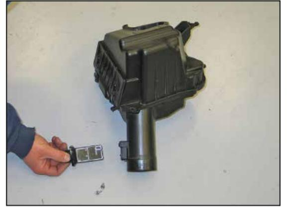
20. Remove the two screws securing the mass air sensor to the driver's side air box and then remove the mass air sensor from the air box.
