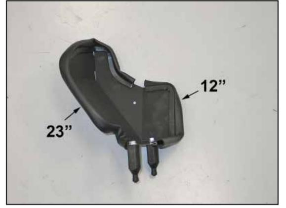
17. Install the trimmed edge trim onto the heat shield as shown.
