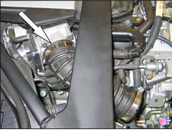
7. Loosen the hose clamp that secures the right side intake tube to the throttle body.
