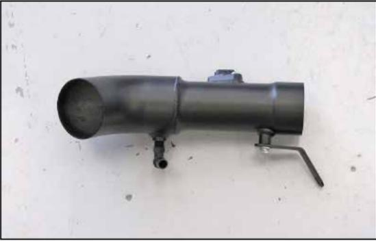
22. Install the tube mounting bracket onto the driver's side K&N® intake tube as shown and secure with the provided hardware.
