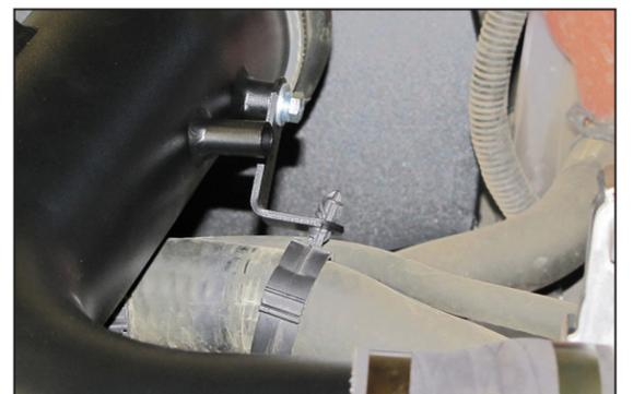
24. Install the upper radiator hose mount onto the mounting bracket installed onto the K&N® intake tube.
