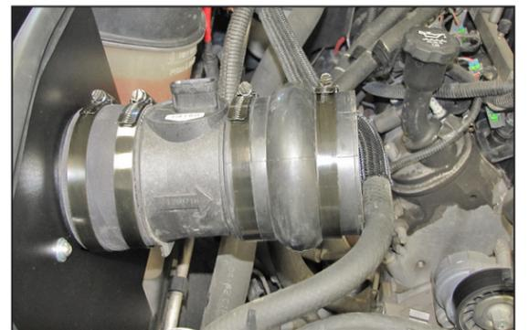
21. Install the silicone hump hose (08543) onto the mass air sensor and secure with the provided hose clamp as shown.
