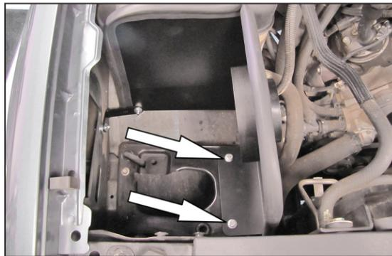
16. Install the heat shield assembly onto the air box-mounting tray and secure to the 5/16" inserted nuts with the provided hardware as shown.
