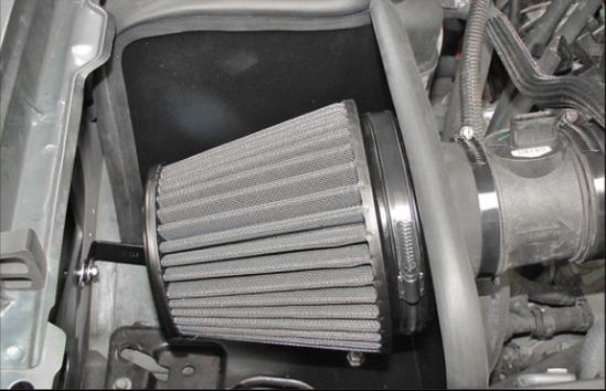
26. Install the K&N® filter as shown and secure with the provided hose clamp.
