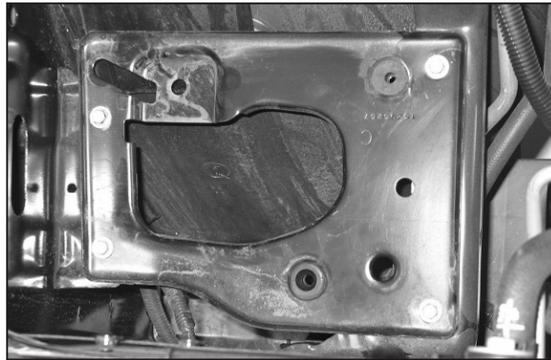
14. Remove the heat shield assembly and drill a 5/8" id hole through the marked location from step #13.
