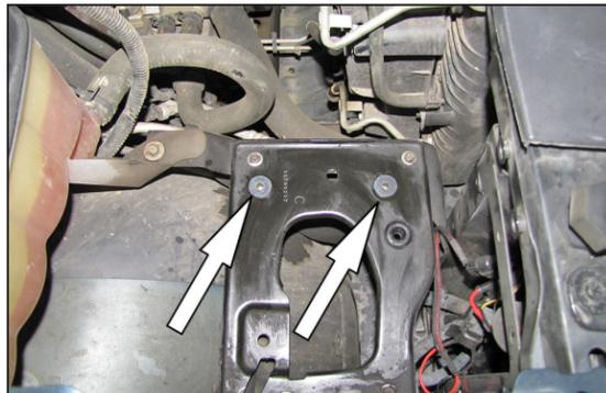
15. Install the two 5/16" inserted nuts into the air box mounting tray as shown.
