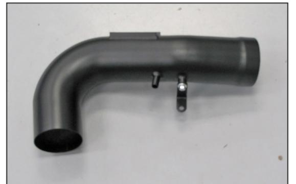
22. Install the "L" bracket (070812) onto the K&N® intake tube with the provided hardware as shown.
