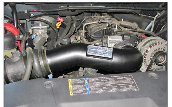
23. Install the K&N® intake tube into the silicone hose at the throttle body and mass air sensor and secure with the provided hose clamps.
