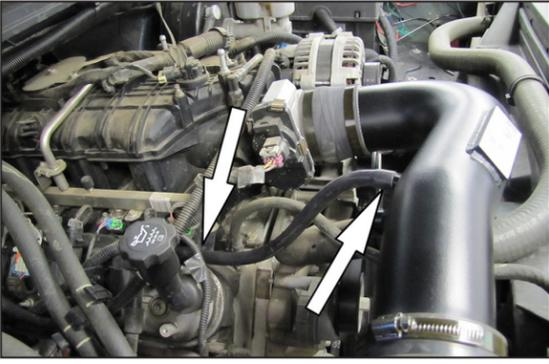
25. Install the provided crank case vent hose onto the valve cover and then onto the K&N® intake tube as shown.
