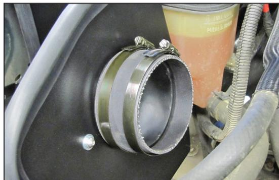
18. Install the silicone hose (08618) onto the filter adapter and secure with the provided hose clamp.
