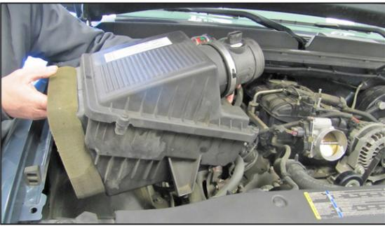
7. Pull firmly upwards to release the air cleaner assembly from the mounting tray grommets, and then remove the assembly as shown.
