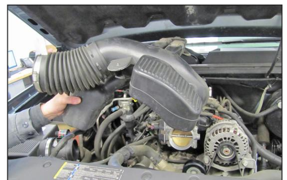
6. Loosen the hose clamps which secure stock intake tube to the throttle body and mass air sensor and then remove the intake tube from the vehicle.
