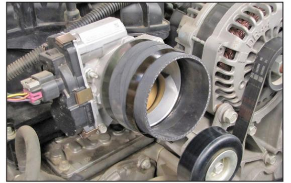
19. Install the silicone (08050) hose onto the throttle body and secure with the provided hose clamp.
