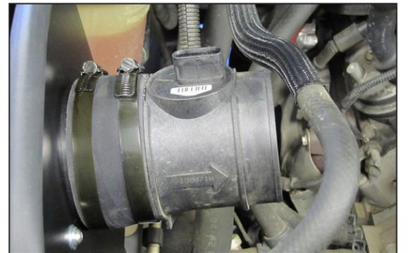
20. Install the mass air sensor assembly into the silicone hose on the filter adapter and secure with provided hose clamp.
