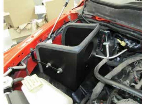
19. Install the heat shield assembly into the vehicle and secure to the bracket previously installed, to the inner fender and rubber mounted stud.
