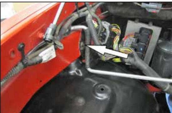
12. Remove the bolt shown which secures the ECU harness bracket to the inner fender.
