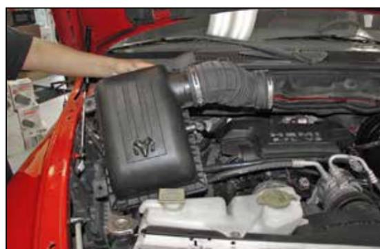
4. Lift up and remove the air filter housing and intake tube from the vehicle.
