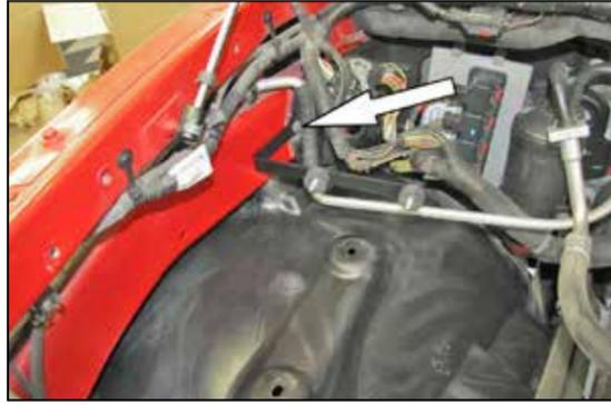
14. Install the bracket assembly onto the inner fender and secure with the bolt removed in step #12.
