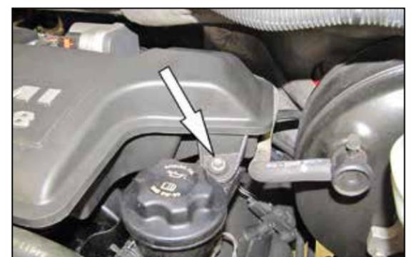
6. Loosen the remaining bolt securing the intake plenum.
