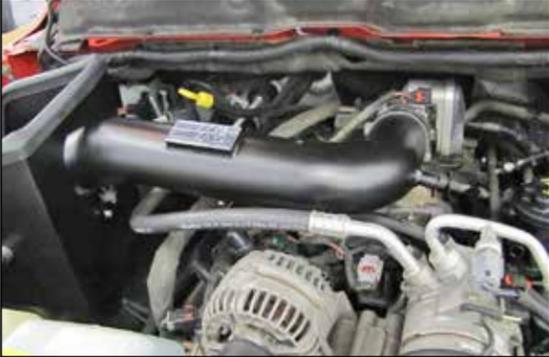
26. Install the intake tube into the heat shield and coupling hose at the throttle body then secure the tube with the hose clamp and hardware,
