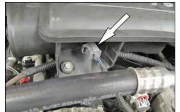
5. Disconnect the inlet air temperature sensor and loosen the bolt securing the intake plenum.
