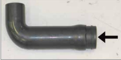
26. On vehicles equipped with an air injection system, install the provided coupler into the cut piece of air injection hose.
