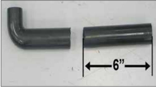
25. On vehicles equipped with an air injection system, cut 6" off of the provided air injection hose as shown.
