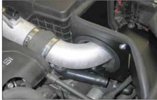
28. Install the provided silicone hump hose (08696) onto the K&N® primary intake tube and then install the primary intake tube into the heat shield. Secure the intake tube with the hose clamps and hardware provided to the mounting bracket and then connect the air injection hose to the factory air injection hose if equipped.
