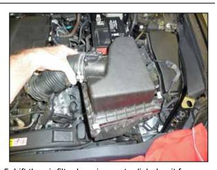
5. Lift the air filter housing up to dislodge it from the mounting grommets and remove the complete assembly from the vehicle.
