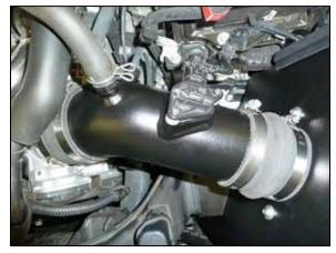
13. Install the intake tube into the previously installed couplers, adjust the tube for best fit and secure with the provided hose clamps. Reconnect the mass air sensor electrical connection. Connect the vacuum line and crank case vent line to the K&N® intake tube.
