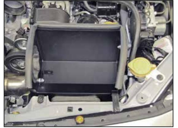
17. Set the heat shield into position on the core support and secure with the factory air box mounting bolts and to the previously installed bracket with the hardware provided.
