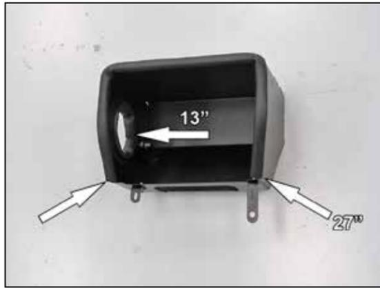
15. Install the 13" long section of edge trim into the hole of the heat shield as shown and then install the 27" long section of edge trim onto the top of the heat shield as shown.
