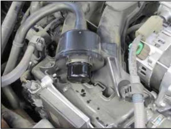
23a. Install the provided caplug onto the engine sound drum as shown.
