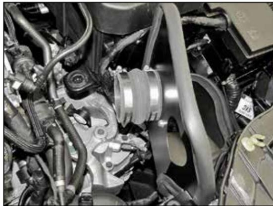
14. Install the provided coupler hose (087212) onto the filter adapter and secure with the provided hose clamp.
