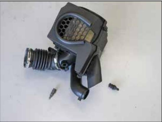
11. Remove the inlet air temperature sensor and mounting post from the factory air box.
