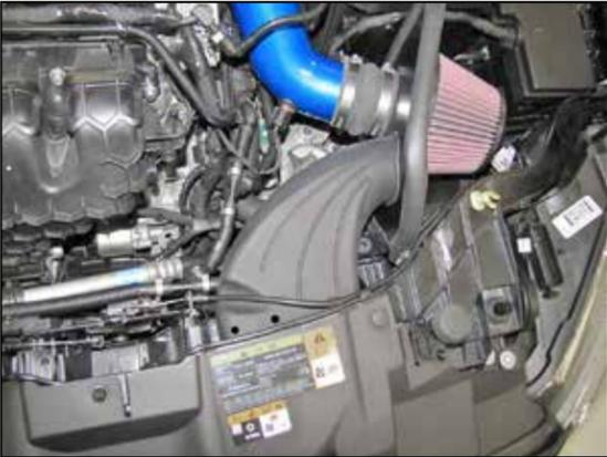
24. Install the K&N® fresh air duct into the heat shield and core support as shown and secure with the two provided retaining clips.
