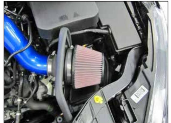
19. Install the K&N® air filter onto the filter adapter and secure with the provided hose clamp.
