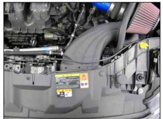
20. Install the K&N® fresh air duct onto the core support and into the K&N® heat shield.
