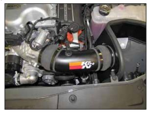
15. Install the K&N® intake tube assembly into position, Slide the coupling hoses out and onto the throttle body and filter adapter. Then adjust the tube and hoses for proper fit and secure with the provided hose clamps.
