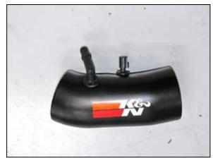
13. Install the crank case vent and inlet air temperature sensor into the K&N® intake tube. NOTE: the inlet air temperature sensor is very fragile, use care while installing the sensor. NOTE: On vehicles with the crank case vent solenoid valve, install the provided 90° vent fitting in place of the factory fitting.
