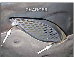
18. If the vehicle is to be driven during inclement weather it is recommended the shield be installed onto the hood vent to guard, the air filter from concentrated water. Remove the two bolts that secure the factory vent grid.
