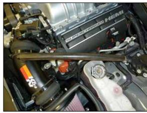
16a. On models equipped with the solenoid vent valve, install the provided crank case vent line and secure to the solenoid vent valve port using the provided hose clamp.
