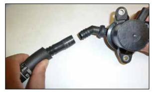
4b. Using a heat gun to warm the nylon vent hose and loosen the connection to the solenoid valve. Disconnect the hose from the solenoid valve.
