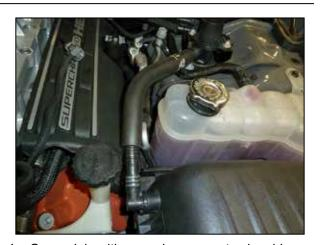
4a. On models with a crank case vent solenoid valve, disconnect the crank case vent line from the solenoid valve on top of the strut tower. Disconnect the shut-off valve electrical connection and then remove the nuts that secure the valve to the mounting bracket. Remove the upper air filter housing and crank case solenoid valve assembly from the vehicle.
