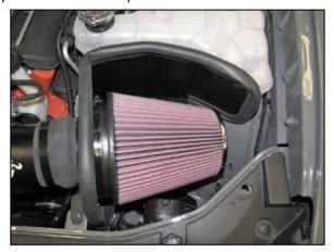
17. Install the  $K\&N^{\otimes}$  air filter and secure with the provided hose clamp.
