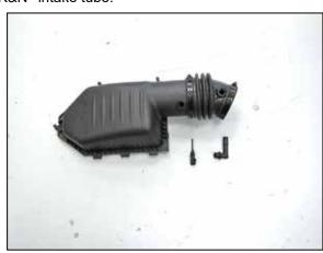
12. Remove the crank case vent and inlet air temperature sensor from the factory intake tube. NOTE: The inlet air temperature sensor is very fragile, use care while removing the sensor.
