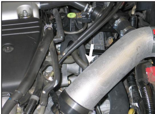
28. Install the stock vent hose onto the K&N® intake tube as shown. Secure with the provided hose clamp.
