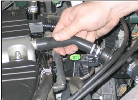
27. Install the crankcase chamber assembly onto the K&N® intake tube and valve cover. Secure with the provided hose clamp.
