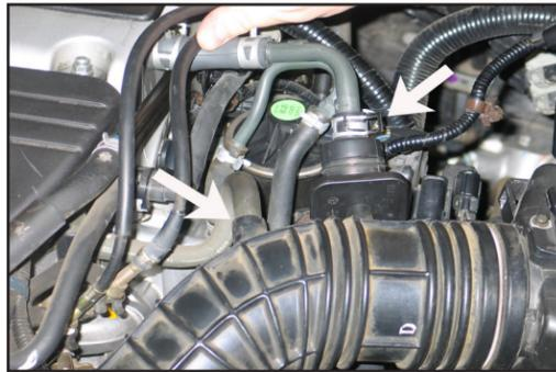
3. Depress the spring clamp and remove the crankcase vent line from the vent chamber on the stock intake tube. Disconnect the vent hose from the stock intake tube.
