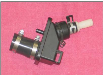
25. Insert the hose mender into the crank case vent chamber. Secure using the stock clamp removed in step # 3.
