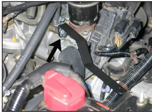
13. Install intake tube bracket (#06498) onto the thermostat housing with the provided hardware as shown.
