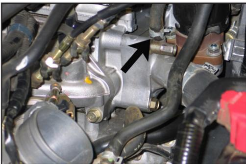
9. Depress the spring clamps on the stock coolant hose at the throttle body and thermostat housing.
