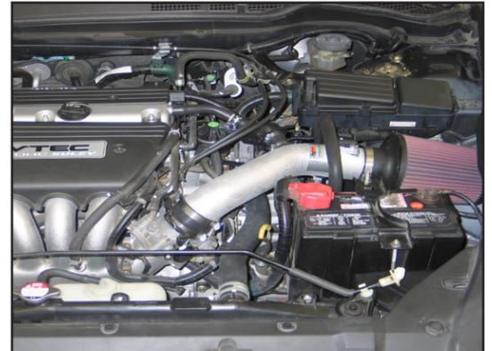
31. Reconnect the vehicle's negative battery cable. Check to ensure all hose clamps and fittings are properly tightened and positioned correctly before starting the vehicle.
