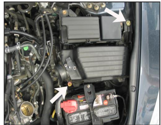
6. Remove the two bolts securing the stock airbox to the vehicle.
