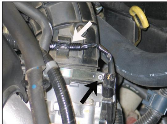
4. Loosen the hose clamp at the throttle body and unclip the throttle position sensor harness from the stock intake tube.
