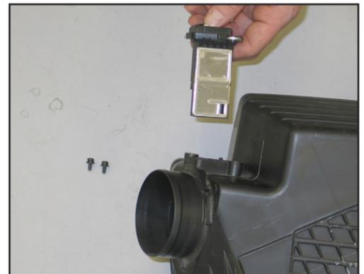
19. Remove the mass air sensor from the stock airbox.
