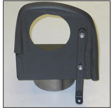
17. Install "L" bracket (#06499) onto the heat shield with the provided hardware as shown.
