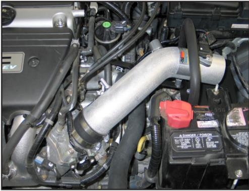
22. Install the K&N® intake tube into the silicone hose at the throttle body and align with the tube mounting bracket installed in step # 13. Secure with the provided hardware and hose clamp.
