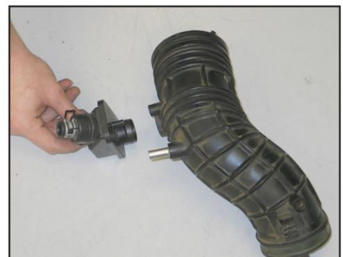
20. Depress the spring clamp and remove the crankcase vent chamber from the stock intake tube.
