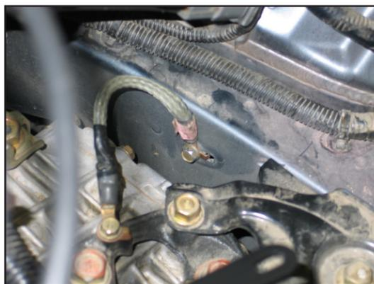
14. Remove the bolt securing the ground strap to the frame rail.
