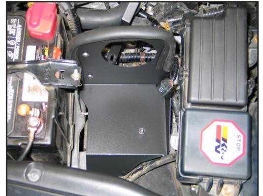
18. Install the heat shield assembly with the provided hardware as shown.
