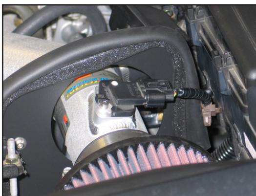
30. Re-connect the mass air sensor connector as shown.
