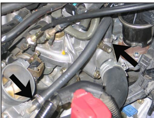
11. Install the supplied coolant hose onto the thermostat housing and throttle body. Secure with the provided clamps as shown.
