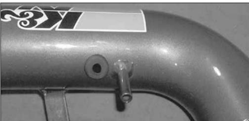
16. Install the provided grommet into the hole on the K&N intake tube as shown.
