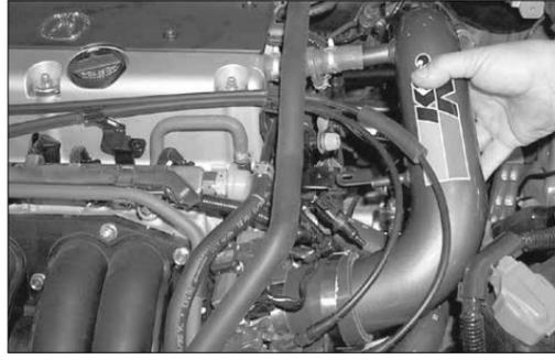
17. Slide the K&N intake tube into the silicone hose on the throttle body, then line up the bracket on the tube with the original air cleaner mounting point as shown.
