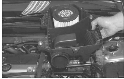
8. Remove the one hex nut and loosen the two hex bolts that secure the lower air cleaner assembly, then remove the assembly as shown.
