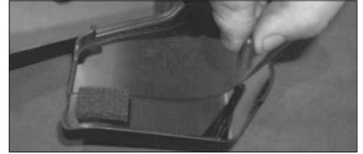
24. Install the rubber cap plug onto the stand-off on the engine cover as shown.
