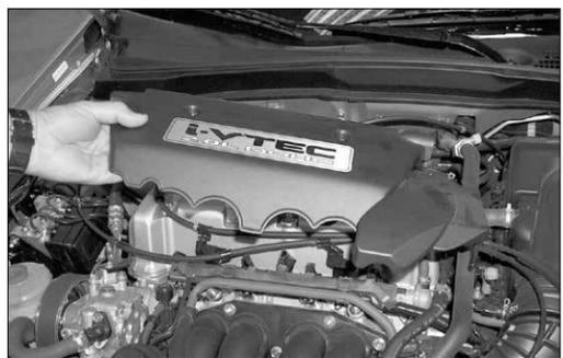
2. Loosen and remove the two bolts that secure the engine cover, then remove the engine cover as shown.
