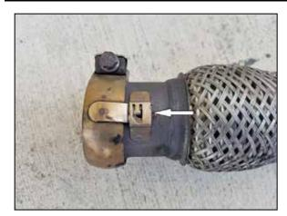
7. Once stock system is removed, remove the conical clamp by prying retaining tang upwards.
