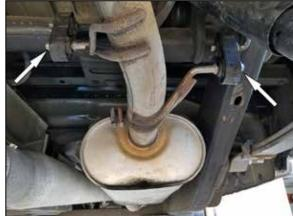
5. Remove muffler assembly from remaining hangers.
