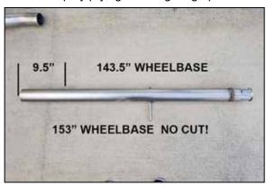
8. For vehicles with 143.5" wheelbase 9.5" must be cut off the end opposite to the conical end connecting to the head pipe (As shown). For vehicles with 153" wheelbase it does not need to be cut.
