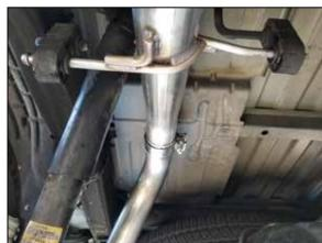
12. Slide band clamp on to the front of the tail pipe section. Then slide tail pipe section into muffler
