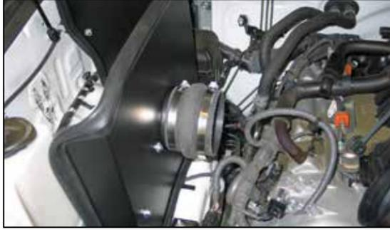
16. Install the silicone hump hose (08418) onto the filter adapter and secure with the provided hose clamp.
