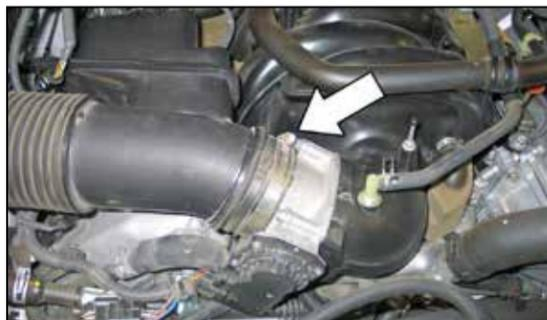
4. Loosen the hose clamp that secures the intake tube to the throttle body.
