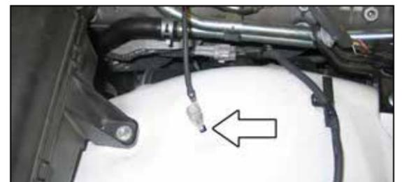
8. Remove the bolt that secures the ground strap to the inner fender.
