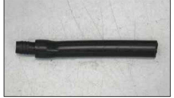
22. Install the hose mender into the provided crank case vent hose as shown.
