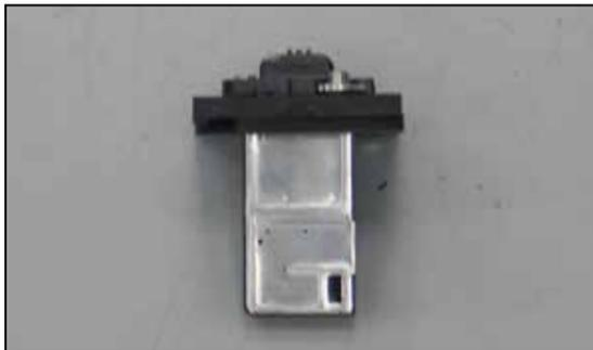
19. Install the mass air sensor through the K&N® mass air sensor adapter as shown. Secure using the provided hardware.
