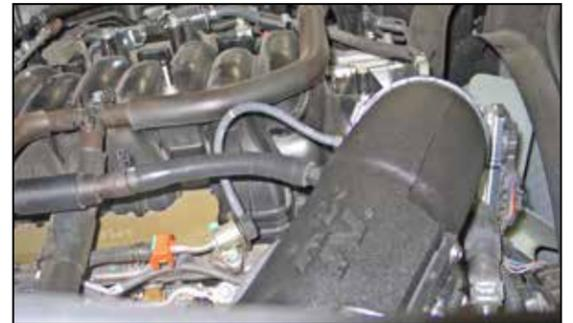
25. Connect the crank case vent hose and the fuel pressure hose to the fittings connected to the K&N® intake tube.
