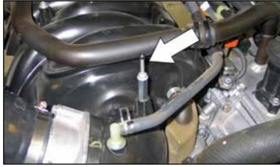
31. Install the factory mounting stud into the nut extension as shown.
