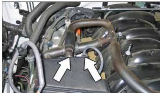
5. Disconnect the crank case vent hose and fuel pressure line from the intake resonator.
