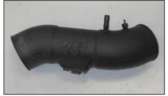
21. Install the provided NPT vent fittings into the K&N® intake tube as shown.
