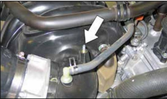
29. Install the provided stud into the mounting stud location as shown.
