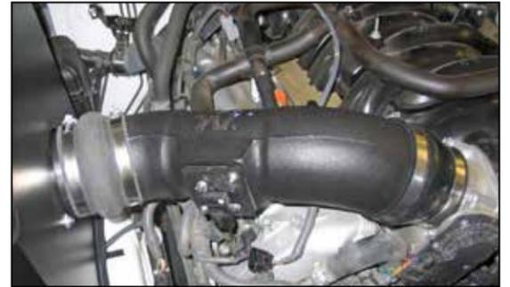
24. Insert the K&N® intake tube into the hump hose attached to the heat shield and then into the step hose attached to the throttle body. Secure with the provided hose clamps.
