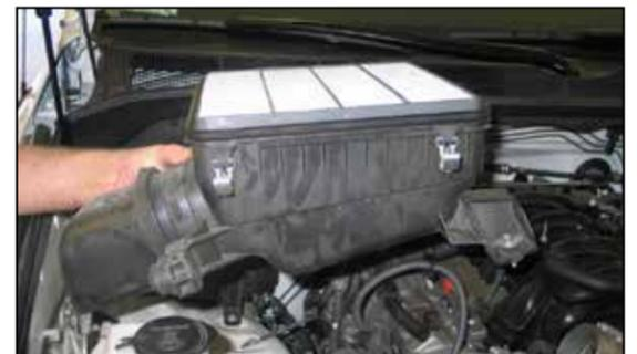
7. Loosen the two bolts securing the lower air box and then remove the lower air box from the vehicle. **NOTE: K&N Engineering, Inc., recommends that customers do not discard factory air intake.**
