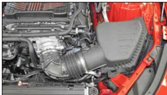
4. Loosen the hose clamp at the throttle body and then remove the complete stock intake system.
