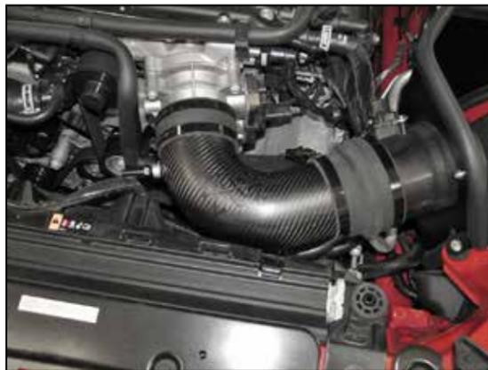
15. Install the K&N intake tube assembly into the hump coupler and then into the coupler at the throttle body, adjust the tube for best fit and then secure with the provided hose clamps.
