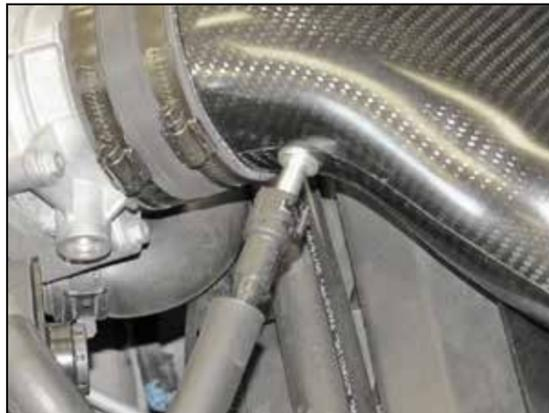
16. Connect the crank case vent tube to the fitting on the K&N® intake tube.
