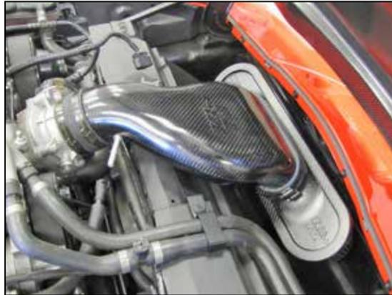
15. Install the K&N® intake system onto the mounting studs, then slide the silicone hose onto the throttle body and secure with the provided hose clamps.
