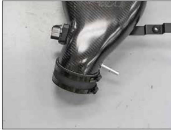
14. Install the provided silicone hose (08761) onto the K&N® intake tube but do not tighten the hose clamps at this time.
