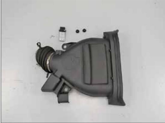
11. Remove the two bolts securing the mass air sensor into the factory intake tube and then remove the mass air sensor. Remove the two factory rubber mounting grommets from the factory intake.
