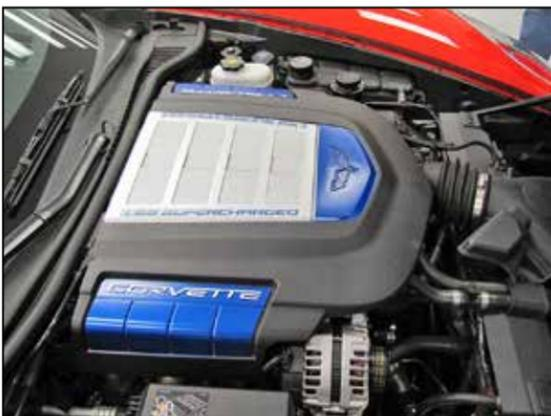
3. Lift up the engine cover to dislodge it from the mounting studs and then remove the engine cover from the vehicle.
