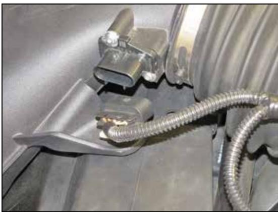
2. Disconnect the mass air sensor electrical connection and unclip the wiring harness from the intake tube.
