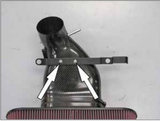
10. Install the tube mounting bracket onto the K&N® intake tube using the provided hardware.
