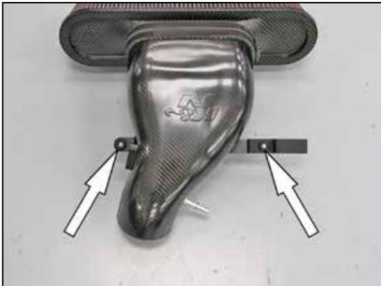
12. Install the factory mounting grommets into the K&N® mounting bracket as shown.
