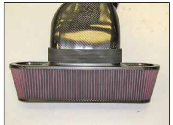
8. Install the intake tube onto the K&N® air filter, slide the silicone hose onto the filter so that it is half on the tube and half onto the filter.
