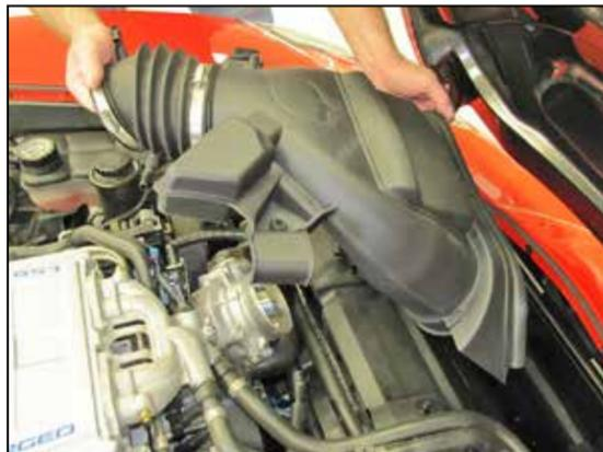
6. Disconnect the intake hose from the throttle body, lift up the intake system to disconnect it from the mounting studs and then remove the intake from the vehicle.
