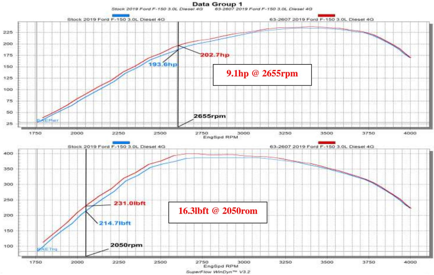
Horsepower gains based on specific or similar vehicle dynamometer test. Results will vary. For more information, lookup vehicle and/or testing protocols at [KNFilters.com](http://KNFilters.com)
