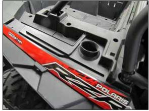
3. Remove the factory prefilters from the vehicle. NOTE: K&N Engineering, Inc., recommends that customers do not discard factory air intake.
