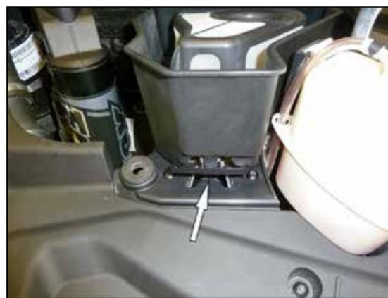
3. Release the locking clip and remove the factory dust filter.
