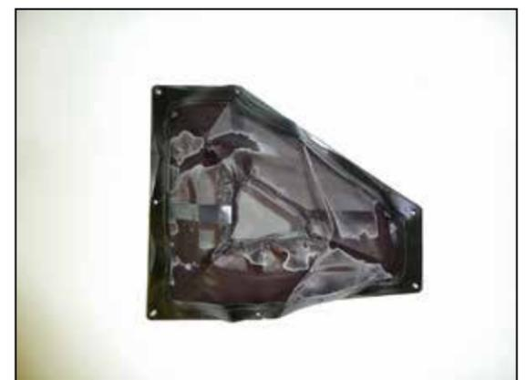
6. Install the K&N® dry charger over the dry charger cage as shown.
