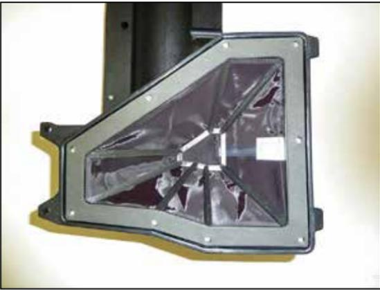
8. Install the provided gasket onto the lower portion of the factory fresh air housing and then install the K&N® fresh air system and secure with the hardware provided.
