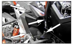
5. Remove the four bolts that secure the right side charger air cooler cover and then remove the cover
