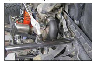
19. Install the K&N® intake tube into the coupler hose and secure with the provided hose clamp. Connect the waste gate vacuum hose to the vacuum switch and secure with the provided tie wrap.
