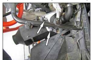
26. Install the factory heat shield onto the K&N® filter assembly then Install the air filter housing assembly, engage the intake tube into the coupler hose and then align the front mounting studs to the factory air filter mounting position. Secure the K&N® housing to the front mounts with the hardware provided. Adjust the intake tube for best fit and then secure all the hose clamps.
