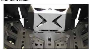
2. Remove the two bolts and nuts shown that secure the cargo tray to the frame.
