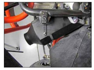
27. Install the provided mounting bracket (083110) as shown using the provided hardware. NOTE: The frame side of the bracket will be secured once the package tray is reinstalled.
