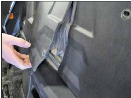
3. Pull back the inner lower corners of the back panels to gain access and remove the two air filter housing mounting bolts.
