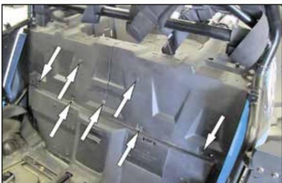
2. Release the locking lever and Remove the (rear) seats from the vehicle and set aside. Remove the eight bolts shown that secure the rear panels.
