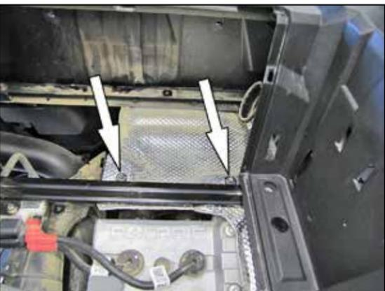
9. Remove the two nuts and bolts shown that secure the heat shielding to the chassis.
