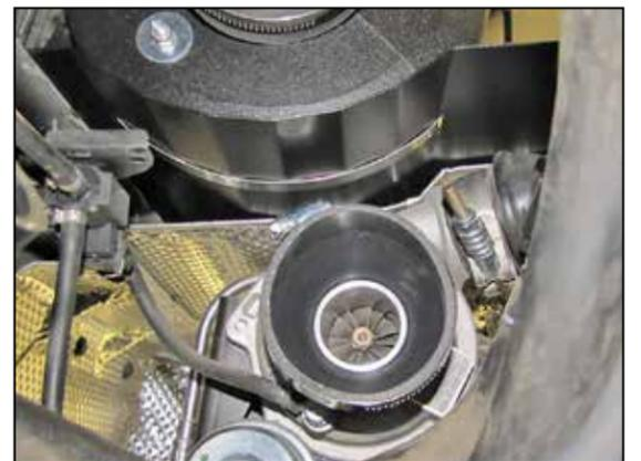
19. Install the provided coupler hose (08667) onto the turbo inlet and secure with the provided hose clamp.
