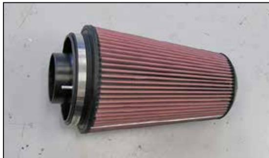
14. Install the adapter assembly into the K&N® air filter and secure with the provided hose clamp.
