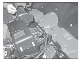
13. Remove the deflector shield as shown.
