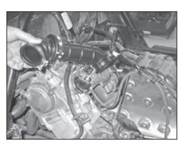
6. Remove the stock intake hose from throttle body and out of the air chamber as shown.
