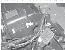
12. Remove the two deflector shield fasteners shown.
