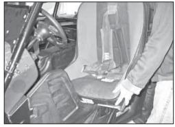
2. Release the locking lever and remove the drivers and passenger seats.
