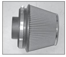
22. Install the provided filter adapter into the K&N® air filter and secure with the provided hose clamp.
