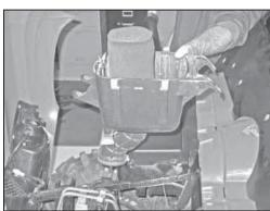
17. Remove the lower air box from the vehicle as shown.
