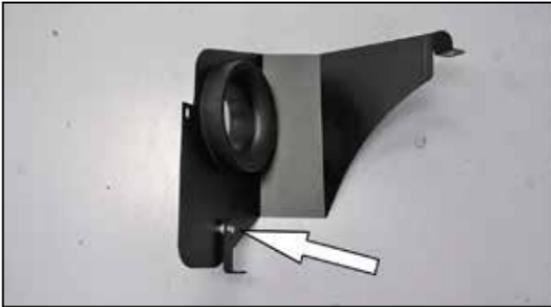
8. Install the heat shield mounting bracket (083170) onto the heat shield and secure with the provided hardware.
