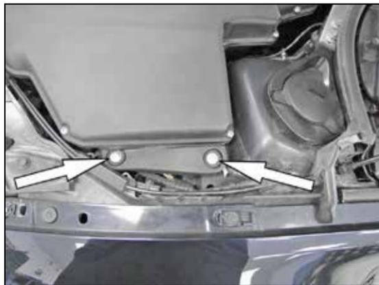
4. Remove the two bolts securing the factory air box to the inner fender.
