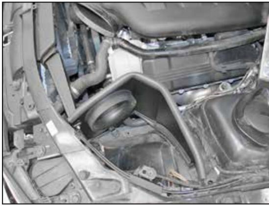
13. Install the fresh air duct onto the heat shield and secure with the provided hardware then install the heat shield assembly onto the air filter housing mounting studs but do not secure at this time.
