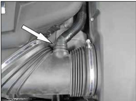
2. Release the locking ring securing the crank case vent to the intake tube and then disconnect the crank case vent hose from the intake tube
