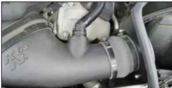
18. Connect the crank case vent hose to the quick disconnect fitting on the K&N® intake tube.
