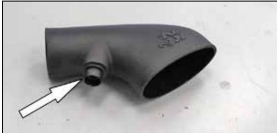
14. Install the provided grommet and quick disconnect fitting into the K&N® intake tube as shown.
