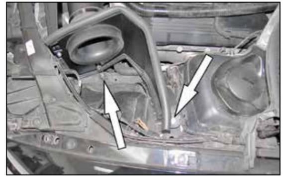
19. Secure the heat shield to the air filter housing studs with the provided hardware.
