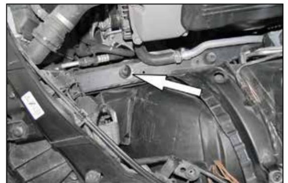
6. Remove the lower air filter mount from the frame rail.
