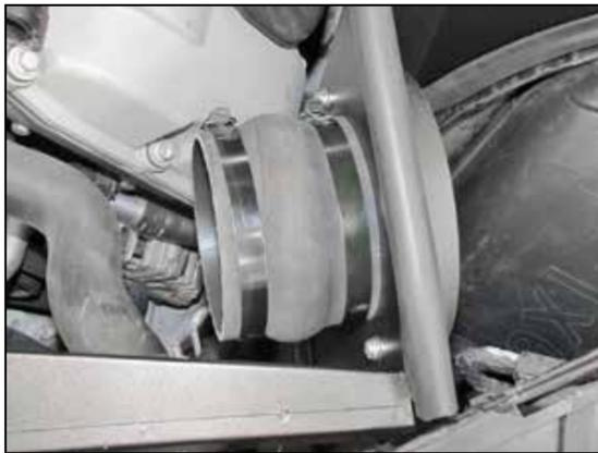
15. Install the provided coupling hose (08418) onto the filter adapter and secure with the provided hose clamp.
