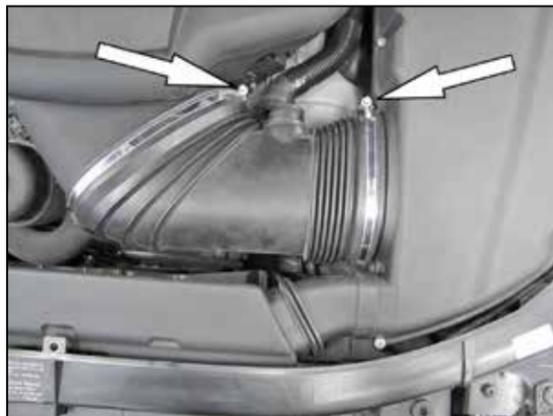
3. Loosen the Hose clamps securing the intake hose and then remove the intake hose from the vehicle.
