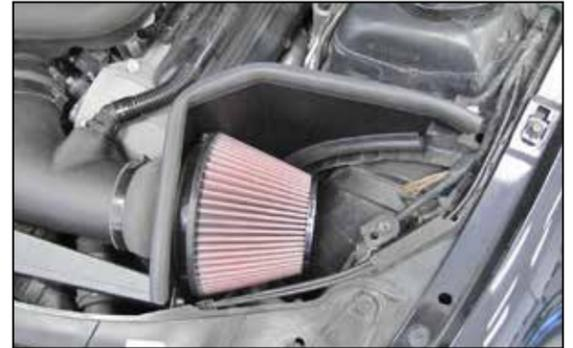
20. Install the K&N® air filter and secure with the provided hose clamp.
