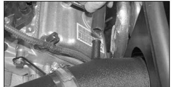
19. Install the provided crank case vent hose onto the vent port on the valve cover then install the vent hose onto the K&N® intake tube. **NOTE: Due to manufacturer changes over time, it may be necessary to use the 5/8 to 1/2 " union fitting and 5/8" CCV hose connected to the 1/2" CCV hose.**
