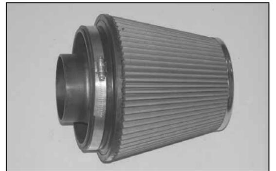
20. Install the filter adapter into the air filter and secure with the provided hose clamp.
