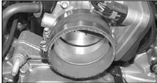
14. Install the silicone hose (08630) onto the throttle body and secure with the provided hose clamp as shown.
