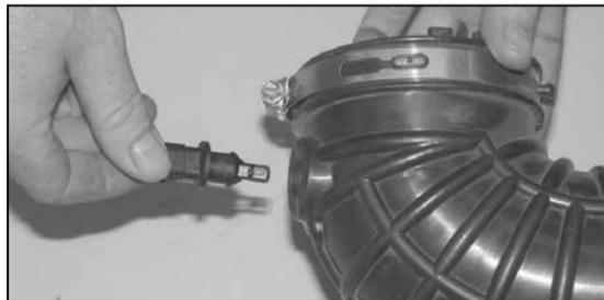
15. Remove the air temperature sensor from the factory intake tube.
