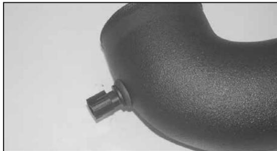
17. Install the factory air temperature sensor into the grommet installed in step #16.
