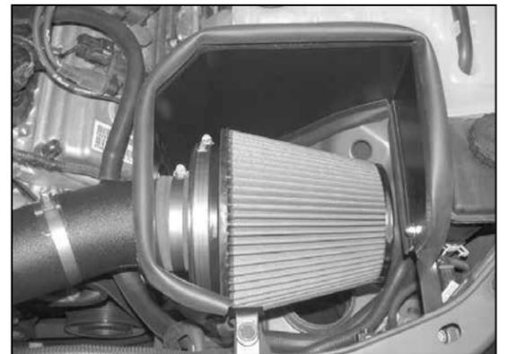
22. Install the air filter assembly onto the K&N® intake tube and secure with the provided hose clamp as shown.
