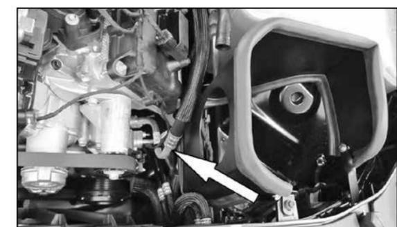
11a. Due to vehicle manufacturing tolerances, the A/C lines on some vehicles may need to be repositioned slightly so that they do not contact the heat shield. To adjust, grab the A/C line on the aluminum section and carefully apply pressure in the desired direction until clearance is obtained.
