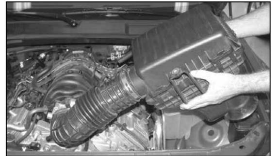
7. Lift the complete intake and air filter assembly to remove it from the vehicle.
