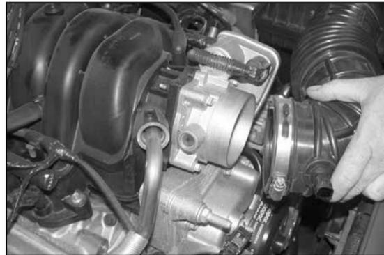
4. Loosen the hose clamp that secures the intake tube to the throttle body and pull the intake tube off of the throttle body.
