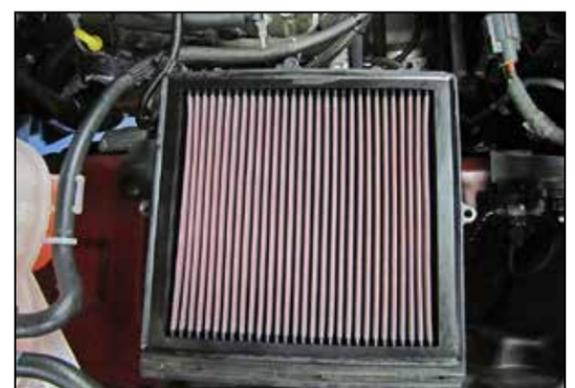
6. Replace the factory air filter with the K&N® air filter provided. Reinstall the upper air filter housing and secure with the factory screws.
