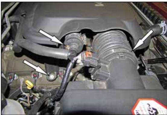
2. Loosen the hose clamp that secures the intake hose to the air filter housing. Using a screwdriver, unlock the small clamp the secures the vent line to the connector and then disconnect the vent line. Remove the bolt securing the intake plenum to the engine.
