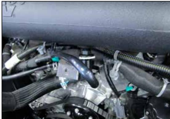
13. Rotate the crank case vent line to line it up with the quick disconnect fitting installed into the K&N® intake tube and then connect the crank case vent.
