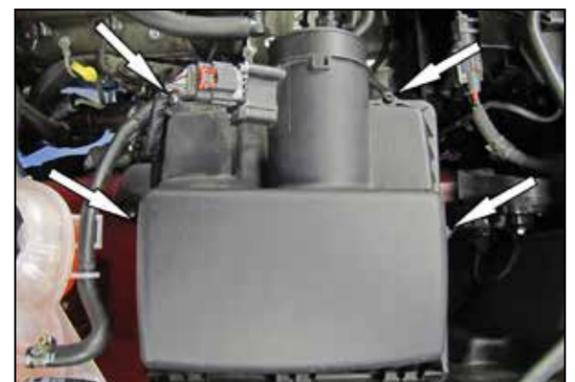
5. Loosen the four screws that secure the upper air filter housing and then remove the upper housing and set aside.
