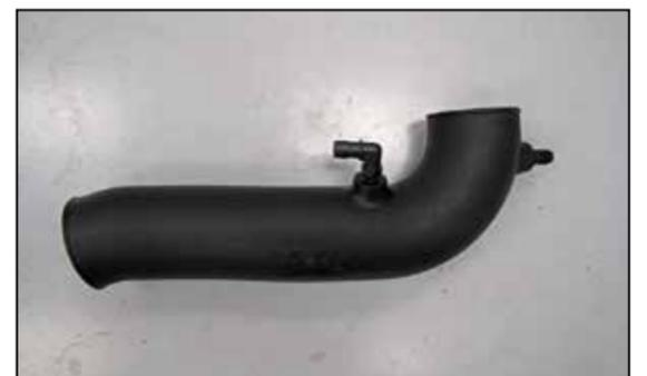
6. Install the provided 90° and straight vent fittings into the K&N® intake tube as shown.
