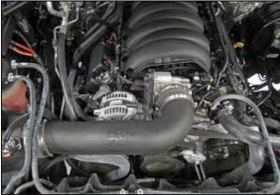
8. Install the intake tube assembly onto the air filter housing and then onto the throttle body, adjust the tube for best fit and then secure with the provided hose clamps.
