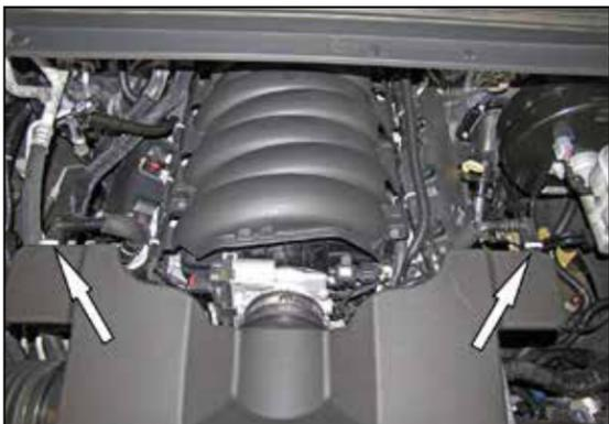
2. Disconnect both crank case quick connect vent lines from the valve covers.
