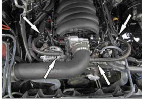
10. Install the crank case vent hose assemblies onto the vent fittings installed into the K&N® intake tube and then connect the quick connect fittings to the port on the valve covers.
