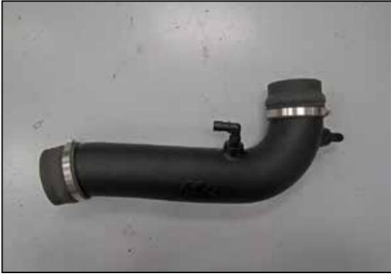
7. Install the provided coupler hoses onto the K&N® intake tube and secure with the provided hose clamps.
