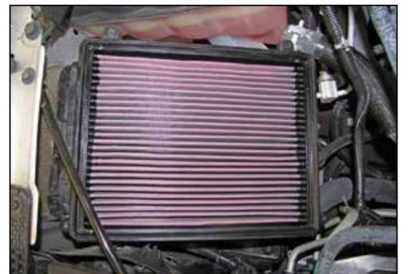
5. Install the K&N® air filter into the lower filter housing and then reinstall the upper housing and secure with the factory hardware.
