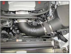
14. Install the K&N<sup>®</sup> intake tube into the hump coupler and then into the coupler at the throttle body, adjust the tube for best fit and then secure with the provided hose clamps.
