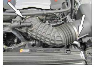
4. Loosen the two hose clamps and then remove the intake tube from the vehicle.
