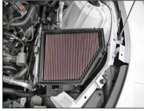
10. Install the provided K&N $^{\mbox{\tiny \$}}$  air filter. Reinstall the lid and secure with the factory screws.
