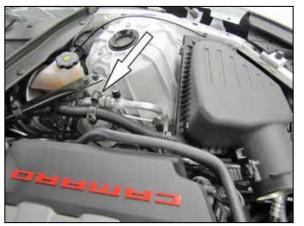
2. Release the spring clamp and then disconnect the sound tube from the intake tube.
