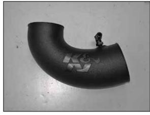
13. Install the provided 90° quick disconnect fitting into the K&N<sup>®</sup> intake tube as shown. NOTE: Plastic NPT fittings are easy to cross
