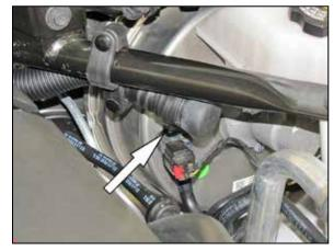
8. Install the union/cap assembly into the rear sound tube.
