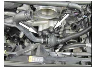
5. Remove the two bolts securing the sound drum to the engine.
