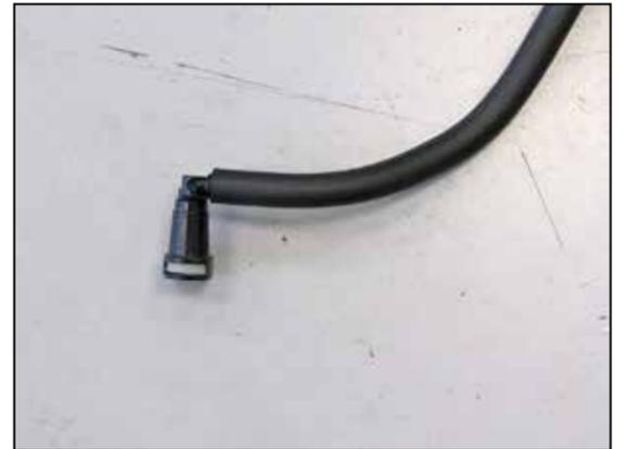
30. Cut the provided crank case vent hose to a length of 15" and install onto the factory 90° quick disconnect fitting.
