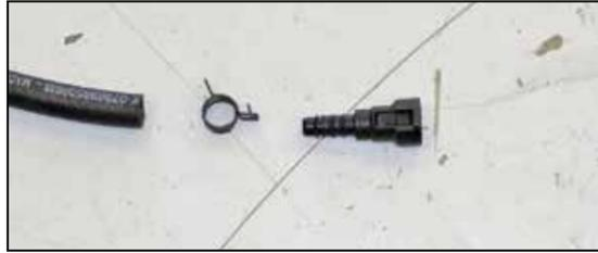
10. Assemble the provided coolant hose (08636), quick disconnect fitting and clamps. Install one clamp 1.5" from the open end of the provided coolant hose.
