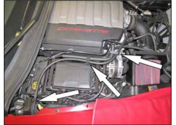
28. On vehicles that are equipped with a "Dry Sump" oiling system, install the crank case vent hose assembly onto the oil tank and then route it through the factory retaining clips and then connect the open end to the 90° fitting installed into the K&N intake tube.
