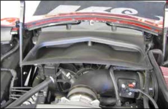
33. Reinstall the air extraction duct and secure with the factory hardware.
