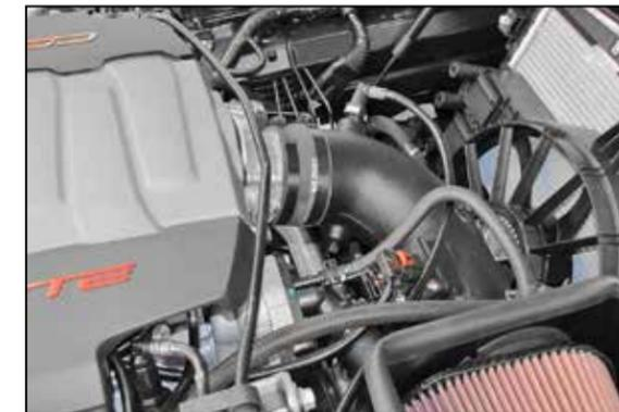
26. Connect the crank case vent hose to the fitting installed into the K&N intake tube as shown.
