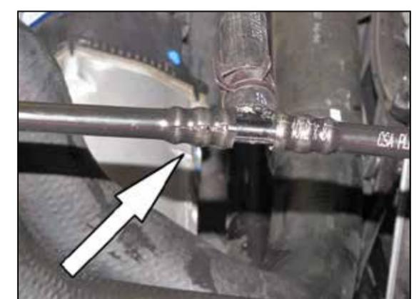
12. Using a razor knife, cut the plastic hose at the TEE fitting where shown. Separate the plastic hose from the TEE fitting.
