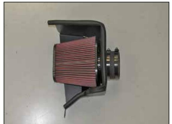
17. Set the air filter into the heat shield and then install the provided coupling hose (08761) onto the filter and secure with the provided hose clamp.
