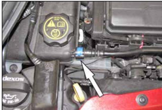
11. **WARNING: Be sure that the engine is cool before proceeding with this step!** Release the blue locking tab securing the factory coolant hose to the expansion tank and then disconnect the hose from the tank.
