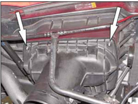
7. Loosen the two TORX fasteners securing the factory mass air sensor housing to the air filter housing and then remove the mass air housing and air filter from the vehicle.
