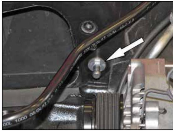
9. Remove the air box mounting stud from the inner fender.
