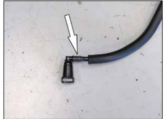
29. On vehicles equipped with a "Wet Sump" oiling system, separate the nylon crank case vent hose from the 90° quick disconnect fitting.
