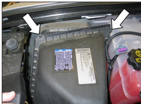
5. Loosen the two screws securing the air box lid and then remove the air box lid and air filter.
