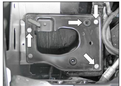
7. Remove the air box mounting grommet and mounting plate bolts shown.
