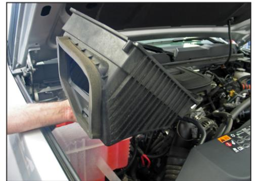
6. Lift up the lower air box to dislodge it from the mounting grommets and then remove the lower air box from the vehicle.
