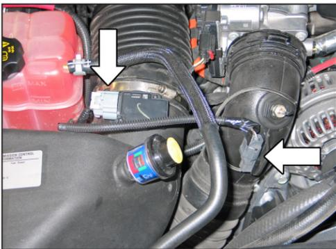
2. Disconnect the mass air sensor and the temperature electrical connection.
