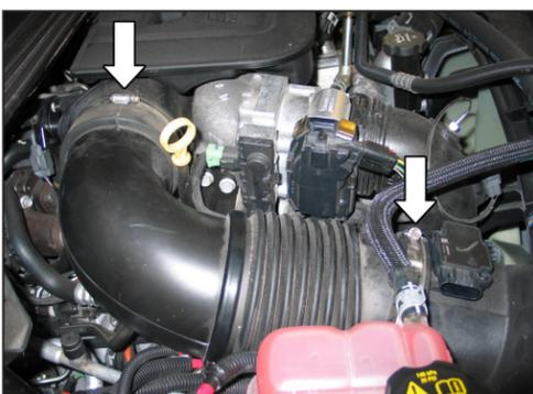
3. Loosen the hose clamps that secure the factory intake tube to the turbo inlet and air box.
