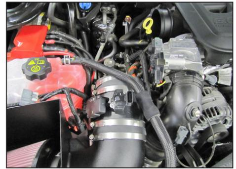
19. Install the mass air sensor assembly onto the K&N® intake tube as shown and secure with the provided hose clamp.
