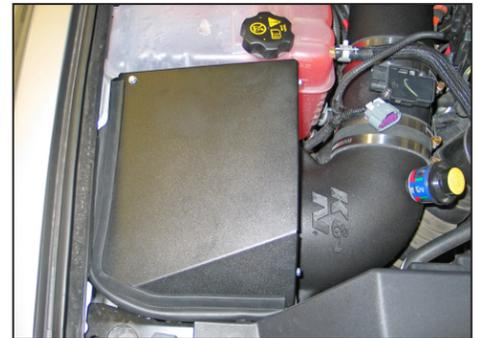
22. Install the heat shield lid onto the heat shield and secure with the provided hardware.
