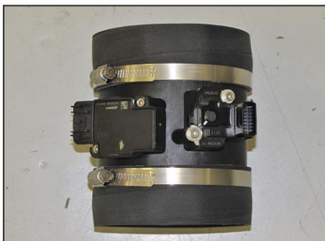
18. Install the two provided silicone hoses (08495) onto the K&N® mass air sensor housing as shown; secure with the provided hose clamps.
