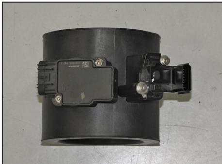
17. Install the mass air sensor into the K&N mass air sensor housing and secure with the provided hardware.
