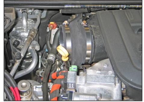
20. Install the provided hump hose (08617) onto the turbo inlet as shown and secure using the provided hose clamp.
