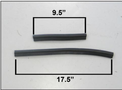
8. Cut the provided edge trim into two sections as shown, one is to be 9.5" long and the other section is to be 17.5" long.
