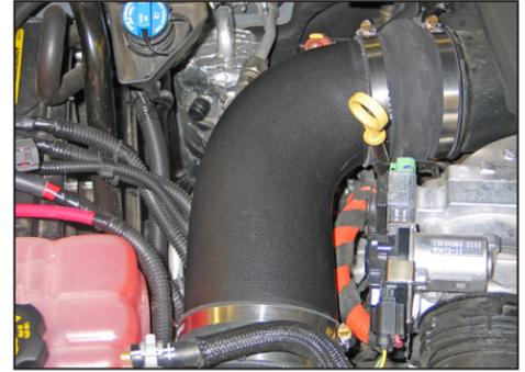
21. Install the K&N® intake tube into the silicone hose at the turbo inlet and then into the silicone hose at the mass air sensor. Adjust the tubes and mass air sensor housing for best fit and then secure with the provided hose clamps.
