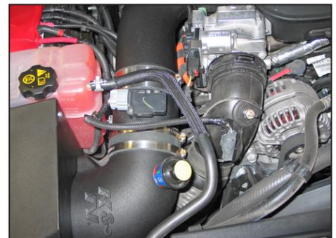
23. Connect the provided MAF extension harness into the factory wiring harness and then connect the open end to the MAF sensor. On models equipped with the second sensor, reconnect the electrical connection at this time also.
