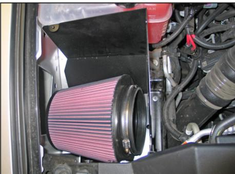
12. Carefully set the K&N® air filter into position on top of the air box tray.
