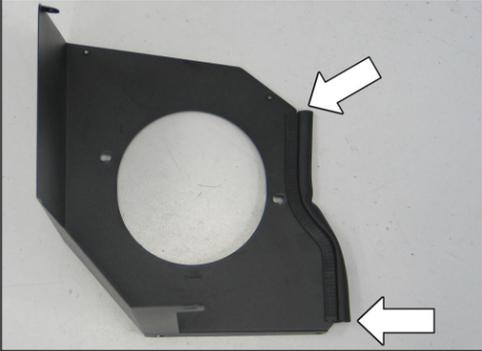
9. Install the 9.5" long section onto the heat shield as shown.
