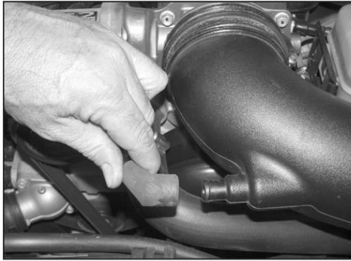
4. Disconnect the crank case vent hose from the factory intake tube as shown.
