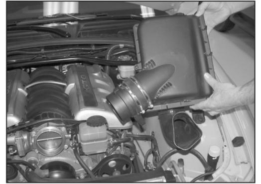
7. Pull up on the air box assembly to dislodge it from the three mounting pins and then remove the air box from the vehicle as shown.
