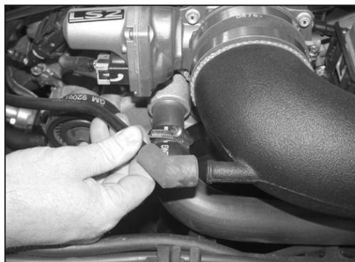
19. Install the crank case vent hose onto the K&N® intake tube as shown.
