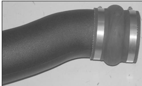
17. Install the silicone hump hose (08176) onto the intake tube as shown and secure with the provided hose clamps as shown.
