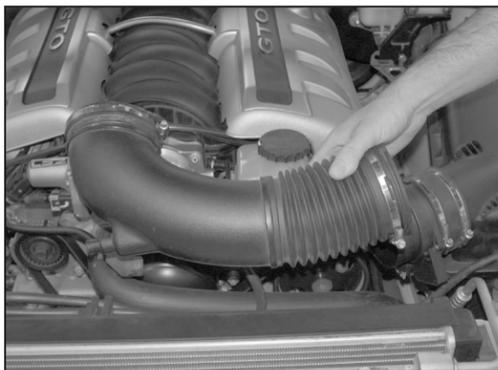
5. Loosen the two intake tube hose clamps, then remove the intake tube from the vehicle.
