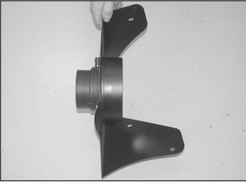
10. Assemble the heat shield and mass air sensor with the provided hardware and gaskets as shown.
