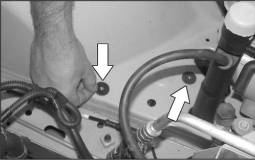
12. Place the two rubber washers onto the inner fender at the lower air box mounting pin locations as shown.
