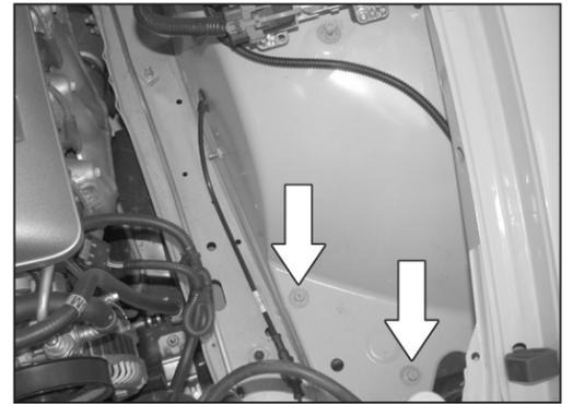
8. Remove the three air box mounting pins shown with a T-30 torx socket.
