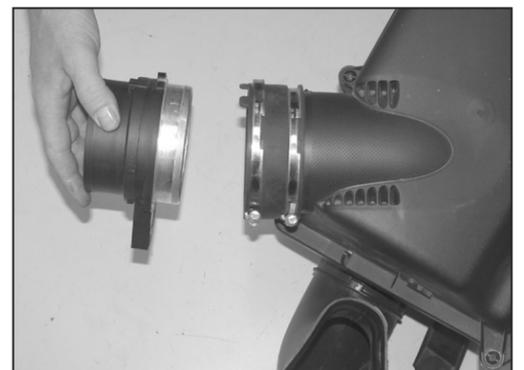
9. Loosen the hose clamp that secures the mass air sensor to the factory air box, then remove the mass air sensor from the factory air box.
