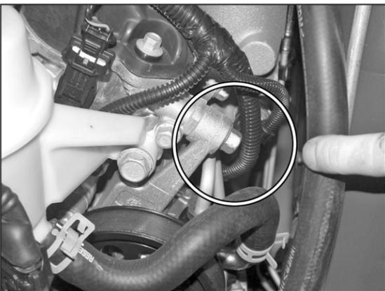
11. Remove the power steering pump mounting bolt shown with a 15mm wrench.
