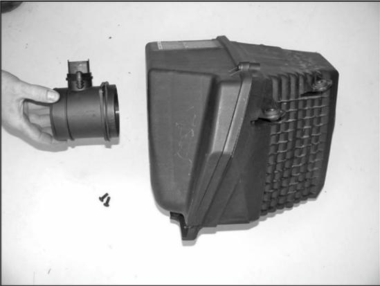
9. Remove the two screws that secure the mass air sensor to the air box, then remove the mass air sensor.
