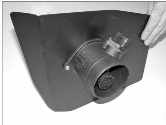
16. Install the mass air sensor onto the heatshield with the provided hardware as shown.
