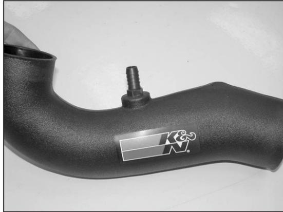
13. Install the provided NPT fitting onto the K&N® intake tube as shown.
