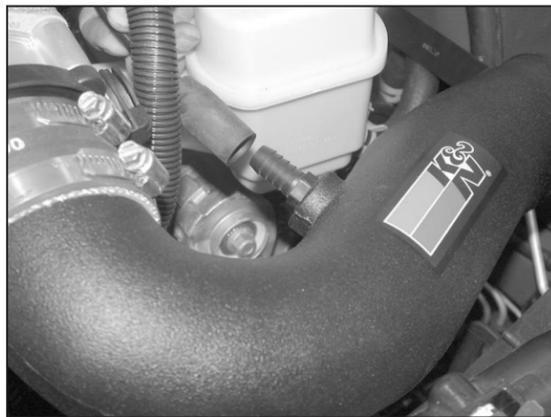
15. Install the crankcase vent hose onto the K&N® intake tube NPT fitting as shown.
