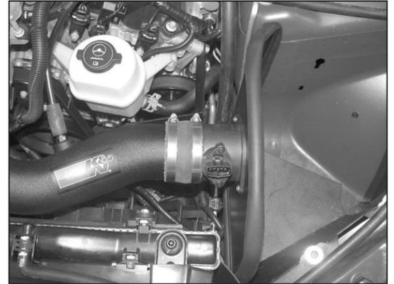
19. Install the heat shield assembly onto the K&N® intake tube and secure with the provided hose clamp.
