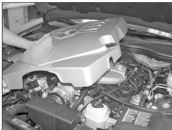
3. Remove oil cap, then pull up on engine cover to release from its retainers.
