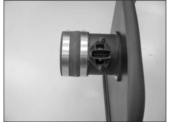
18. Install the silicone hose (#08690) onto the mass air assembly with the provided hose clamps as shown.
