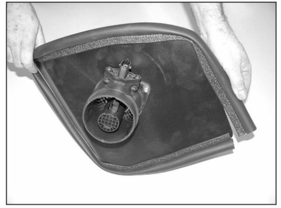
17. Install the edge trim onto the heatshield as shown. Trim if needed.
