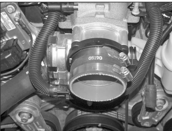
10. Install silicone hose (#08190) onto the throttle body with the provided hose clamps as shown.
