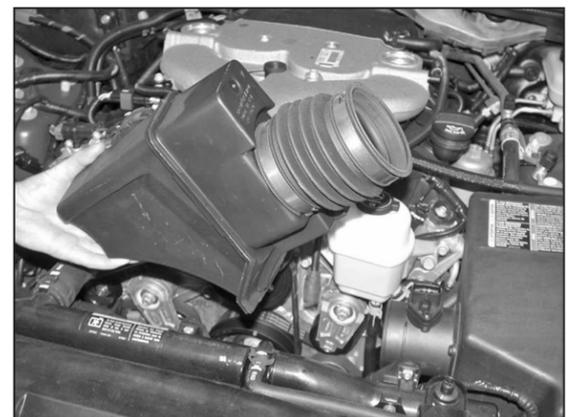
5. Loosen the two hose clamps on the intake plenum, then remove the intake plenum from the vehicle as shown.
