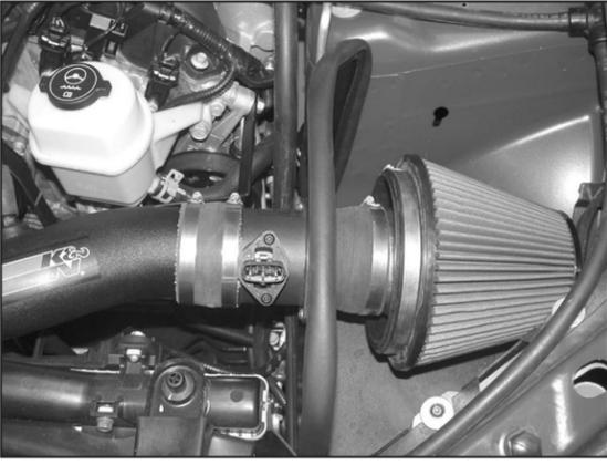
22. Install the filtercharger assembly onto the mass air sensor and secure with the provided hose clamp.
