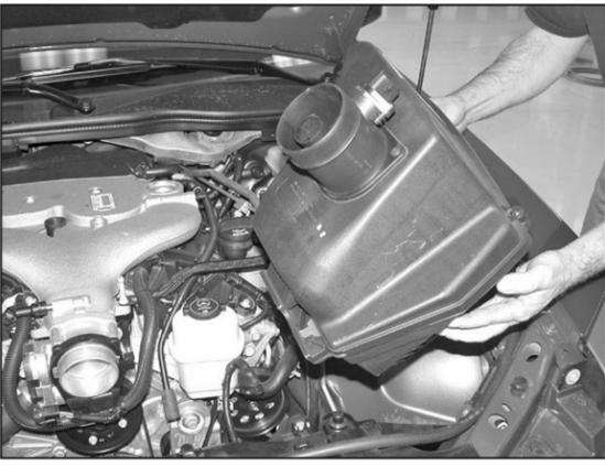
7. Remove the air box from the vehicle as shown.
