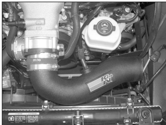
14. Install the new K&N® intake tube onto the throttle body and secure with the provided hose clamp. Secure the tube to the K&N® tube bracket with the hardware provided.
